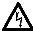
Before you open the TURBOTRONIK, please first ensure that the turbomolecular pump has been braked to a complete standstill, and that the mains power cord is disconnected. Since, nonetheless dangerous voltages may occur the unit must only be opened by a qualified electrician.
