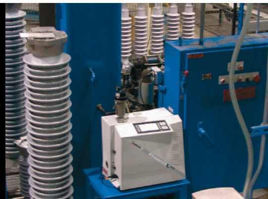
Electrical industry (Photo: Leak test of electrical surge arresters. By courtesy of ABB Inc., Youngwood, PA (USA))
