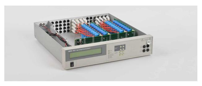
The 964i holds up to 8, eight channel HV switching cards. That's up to 64 test points in a single mainframe - multiple units can be combined to increase capacity
