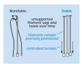
Filament must remain in position over time.
