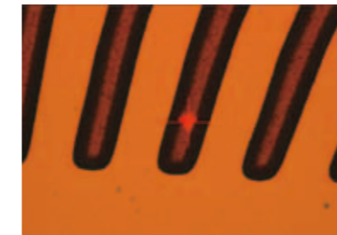
Lead tilt measurement (TTL laser AF) Photos courtesy of: Hirai Seimitsu Kogyo Corporation
