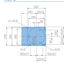
Mounting options: Floor, wall, ceiling Protection class: IP54/67
