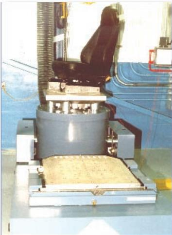
H560B-16 with slip table assembly, and guided head expander, testing an automotive seat track for squeak & rattle noise measurements and key life/durability
