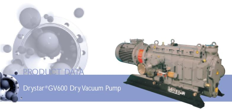
The GV600 dry pump extends the range of the currently successful GV Drystar® series. The pump is based on the well-proven claw mechanism but has an additional roots stage to enhance pumping speed in the working range. This makes it ideal for backing industrial diffusion pumps, without the need for an additional mechanical booster. The higher speed reduces time to crossover pressure.
